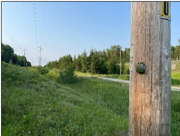
Figure 5. Song Meter Micro autonomous recording unit deployed along the transmission right-of-way, July 2021.
