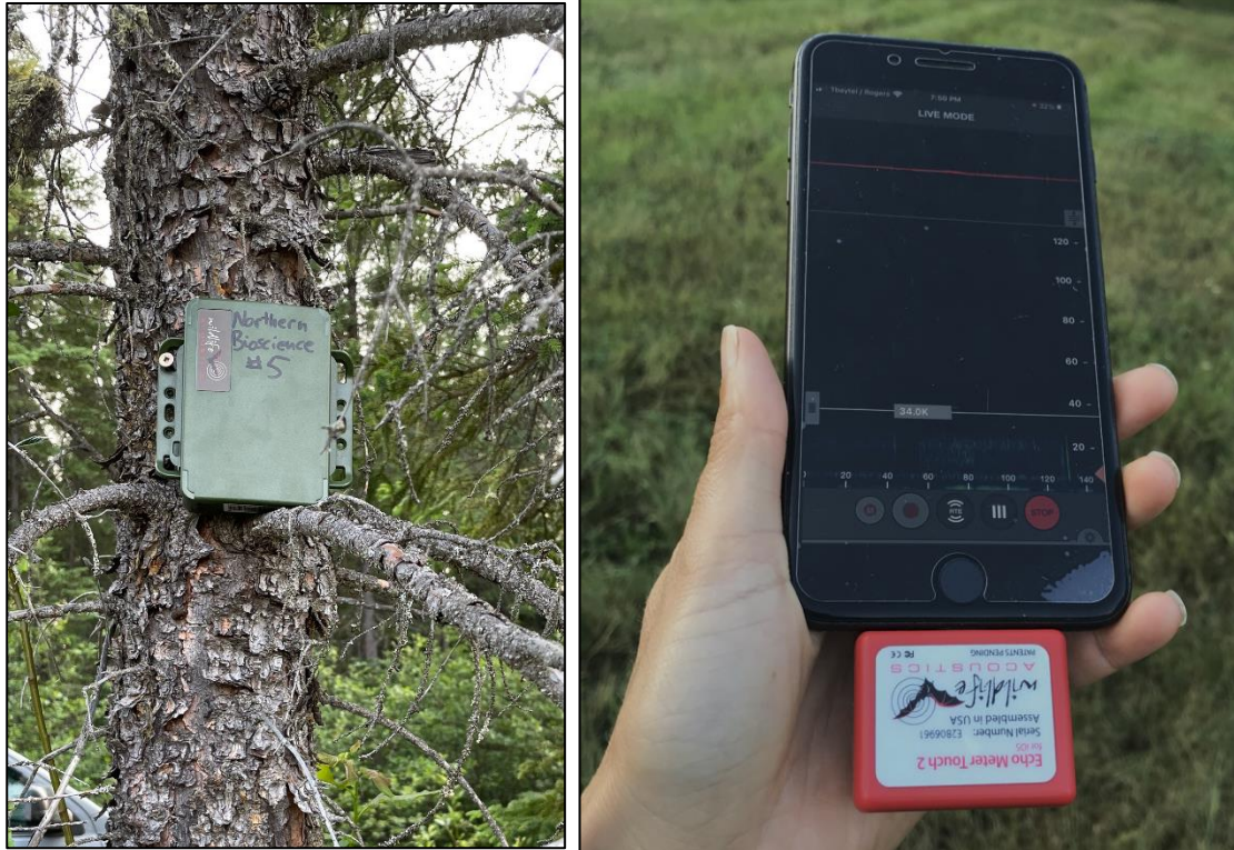
Figure 2. Wildlife Acoustics MiniBat autonomous recording unit (left) deployed for ultrasonic surveys of bats and hand-held Echo Meter Touch 2 (right) used for point-in-time surveys.
