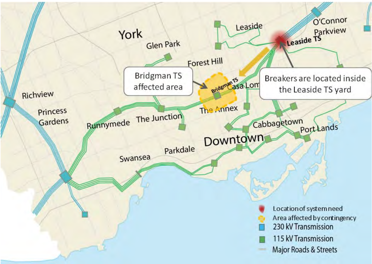
Figure 6-4: Leaside TS Equipment and Affected Areas
