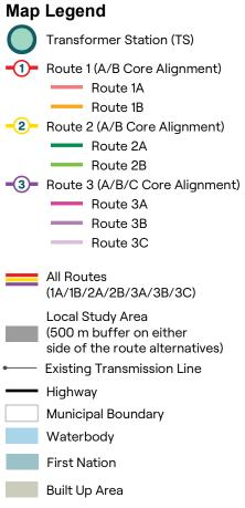
Note: With the exception of the section of Route 3 shown in inset 1, each route represents two transmission lines with parallel alignments. Each line has an assumed 60m right of way, pending detailed engineering.
