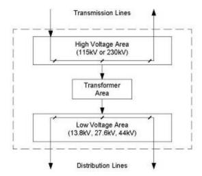
Figure 10: Components of a Typical Simple Transformer Station
