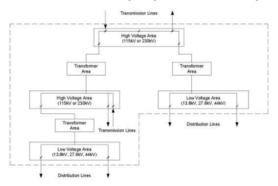
Figure 11: Components of a Typical Complex Transformer Station
