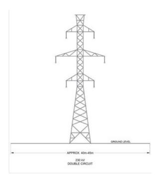
Figure 9: Typical Right-of-Way Width for a 230kV Two-Circuit Transmission Line
