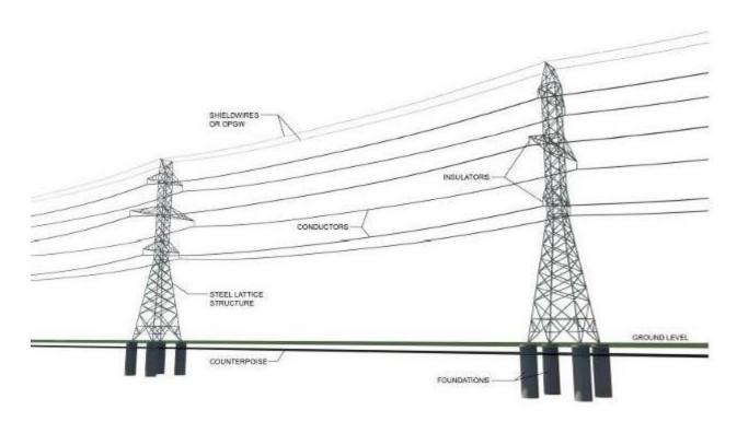
Figure 7: Component Parts of a Typical Transmission Line
