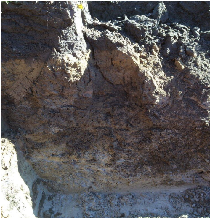
Photo 3: TP2-14 - October 9, 2014 Minor seepage noted at 1.2 m BGS
