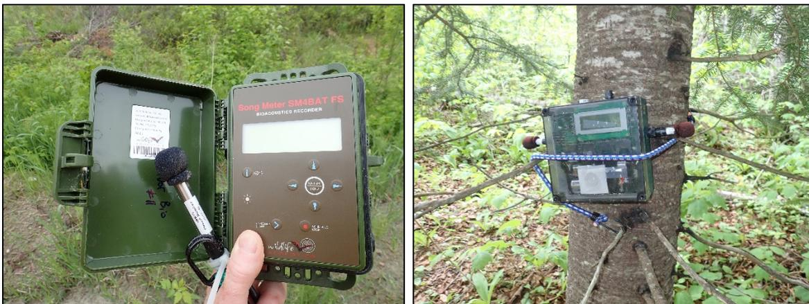
Figure 3. Wildlife Acoustic Song Meter SM4Bat ultrasonic recorder (left) and (right) deployed at the Wawa TS in May-June 2019.
