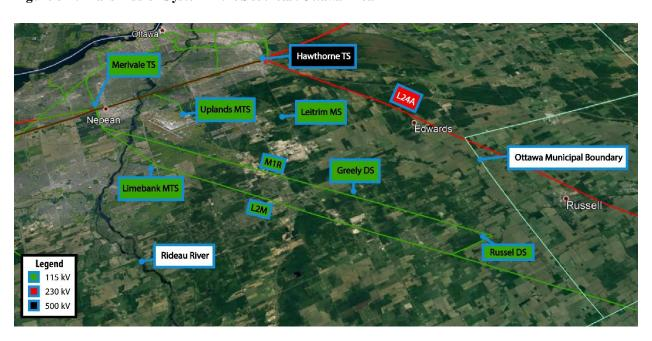
Figure 6-4: Transmission System in the Southeast Ottawa Area
