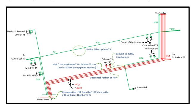
Figure 7-4: Single Line Diagram of the East Ottawa Transmission System if Bilberry Creek TS Were Retired
