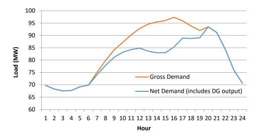
Figure B-1: Sample Profile Before and After Adjusting for Distributed Generation
