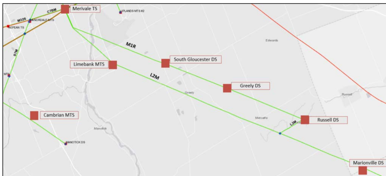
Figure 7-3. Limebank MTS and Marionville DS connection to L2M.
