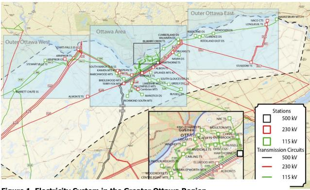
Figure 1. Electricity System in the Greater Ottawa Region
