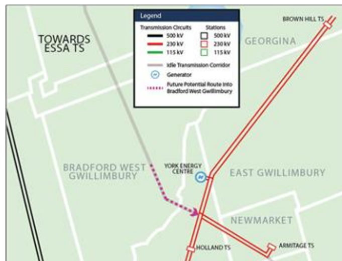
Figure 27: Conceptual Corridor route between Essa TS and Holland Marsh JCT (Courtesy: IESO)
