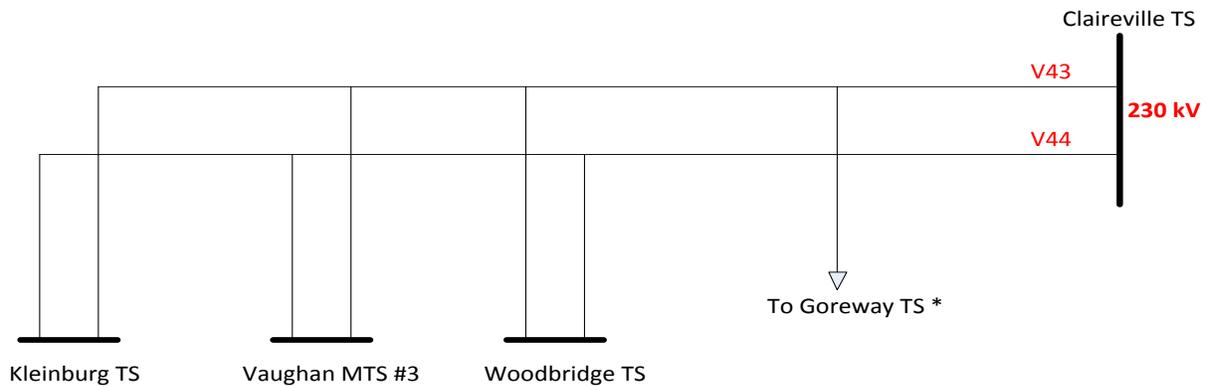
\* Goreway TS is not part of the GTA North, Western Sub-Region study but its loading is considered due to impact on loading of circuit V43.
