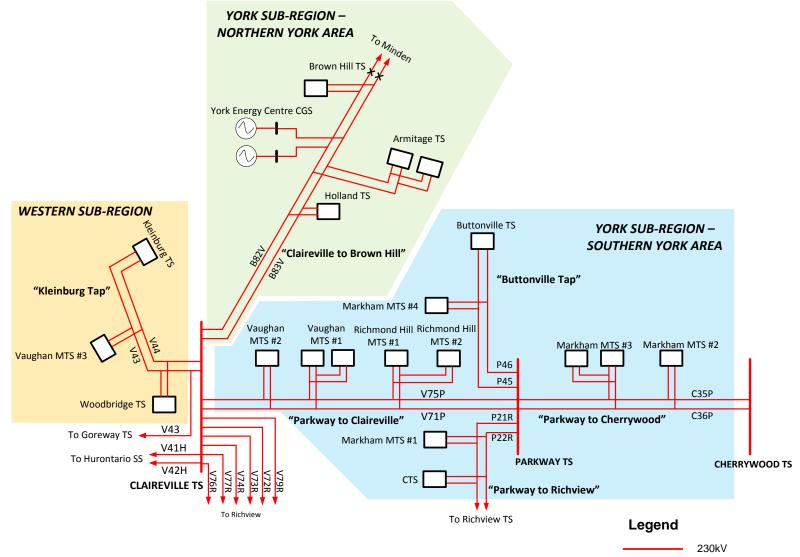
Figure 3-2 GTA North Transmission Single Line Diagram
