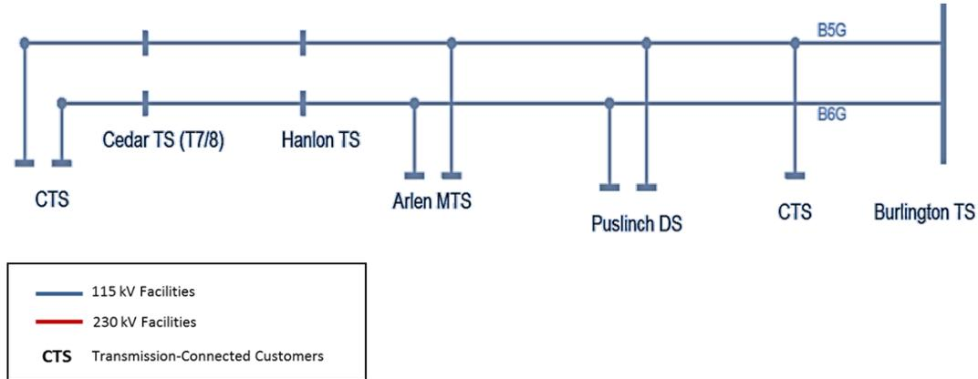
Based on the application of ORTAC criteria, this system has an LMC of 100 MW. This limit is based on the voltage limitations of the B5G circuit, assuming the B6G is out-of-service.
