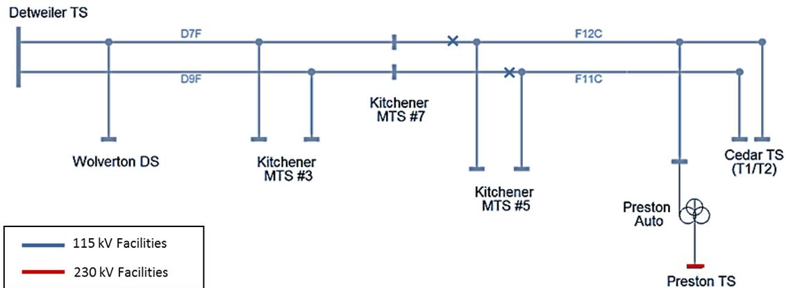
Based on the application of ORTAC criteria, this system has a LMC of 260 MW. This limit is based on the thermal overloading of the D7F circuit, assuming the D9F circuit is out-of-service.
