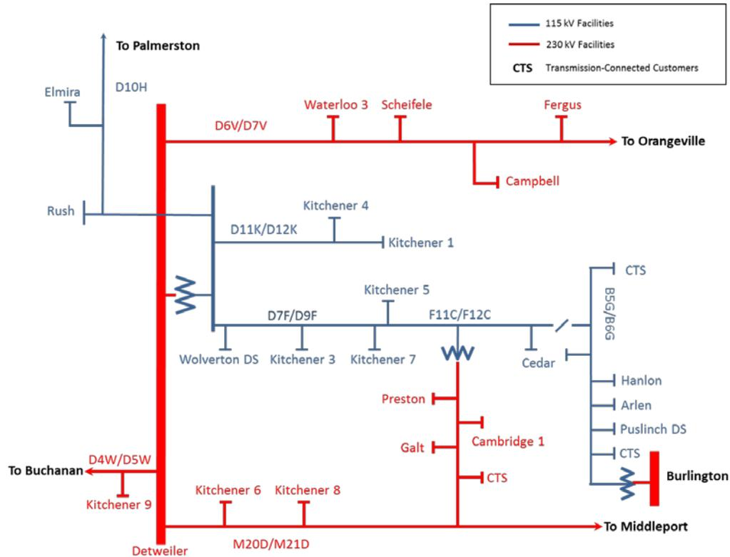
There is no major generation station in the KWCG Region. The majority of supply to the load is provided by a number of 500 kV to 230 kV and 230 kV to 115 kV auto-transformers as follows:
