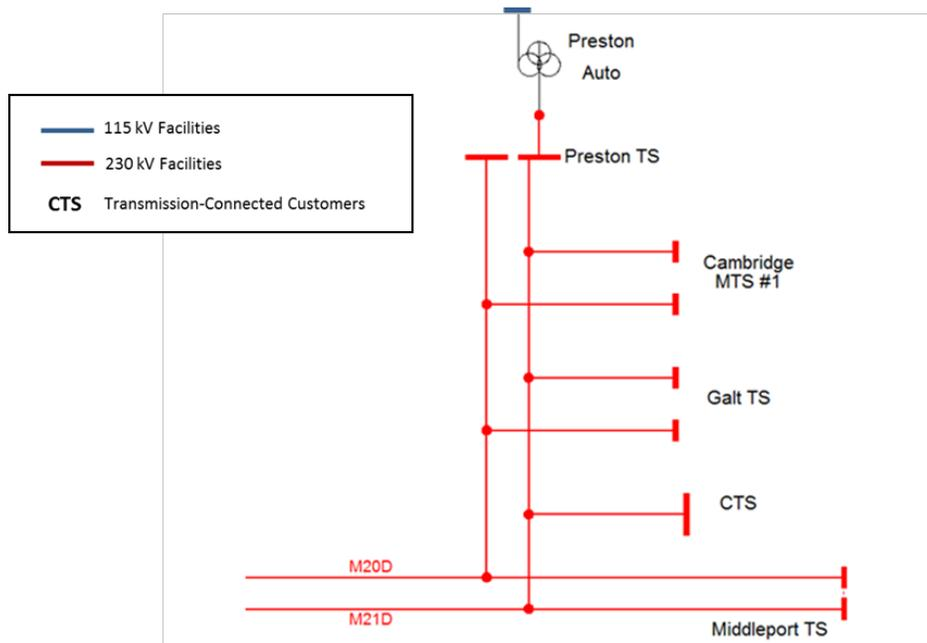
Based on the application of ORTAC criteria, this system has a LMC of 375 MW. This limit is based on the thermal overloading of the M20D circuit, assuming the M21D circuit is out-of-service.
