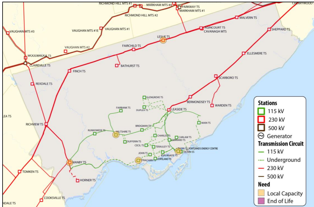
Figure 6-8: Location of Local (Transformer Station) Capacity Needs
