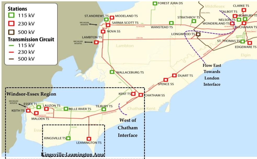
Figure 4-2: The Windsor-Essex Region Electrical Single Line Diagram
