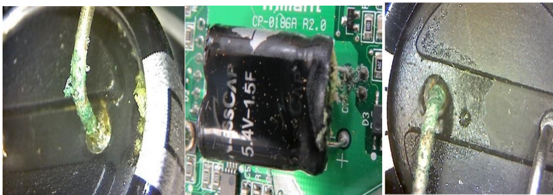
Figure 6: Capacitor Electrolyte Leakage
