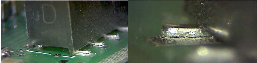
Figure 78: Cracked Solder Joints
