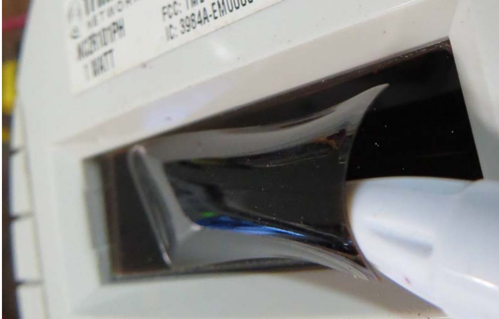
Figure 45. Detached and darkened top polarizing filter
