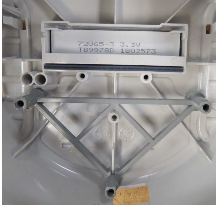
Figure 10. Bracket added to reduce mechanical stress on the connector
