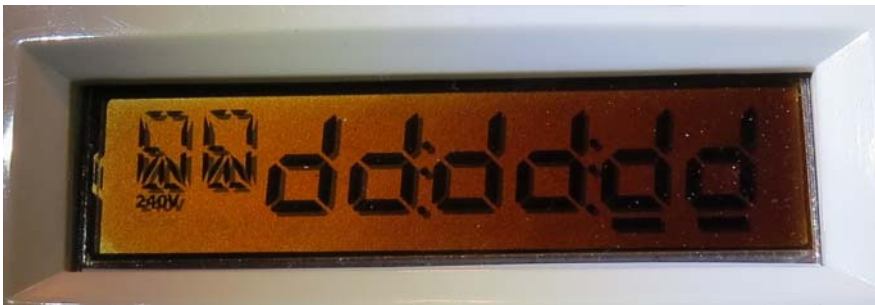
Figure 26. Missing segments on meter J2038889
