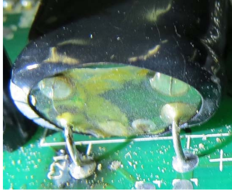
Figure 1. Capacitor C21 failure
