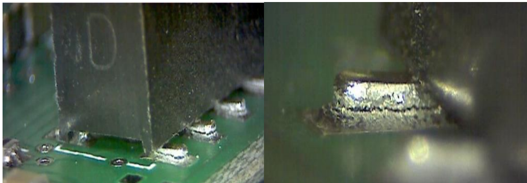
Figure 8: Cracked Solder Joints
