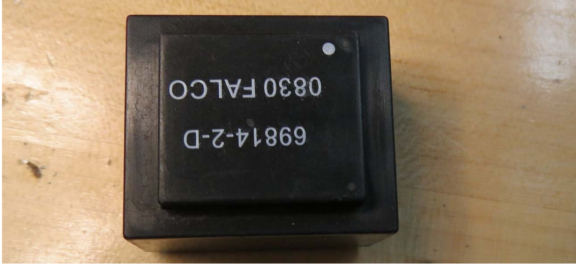
Figure 34. XFO failure on meter #17 – J2965534
