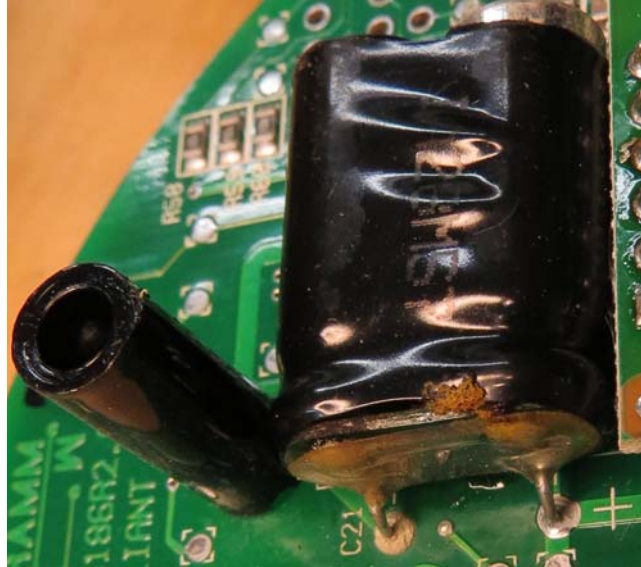
Figure 30. Condition of C21 on meter #10 – J2573411
