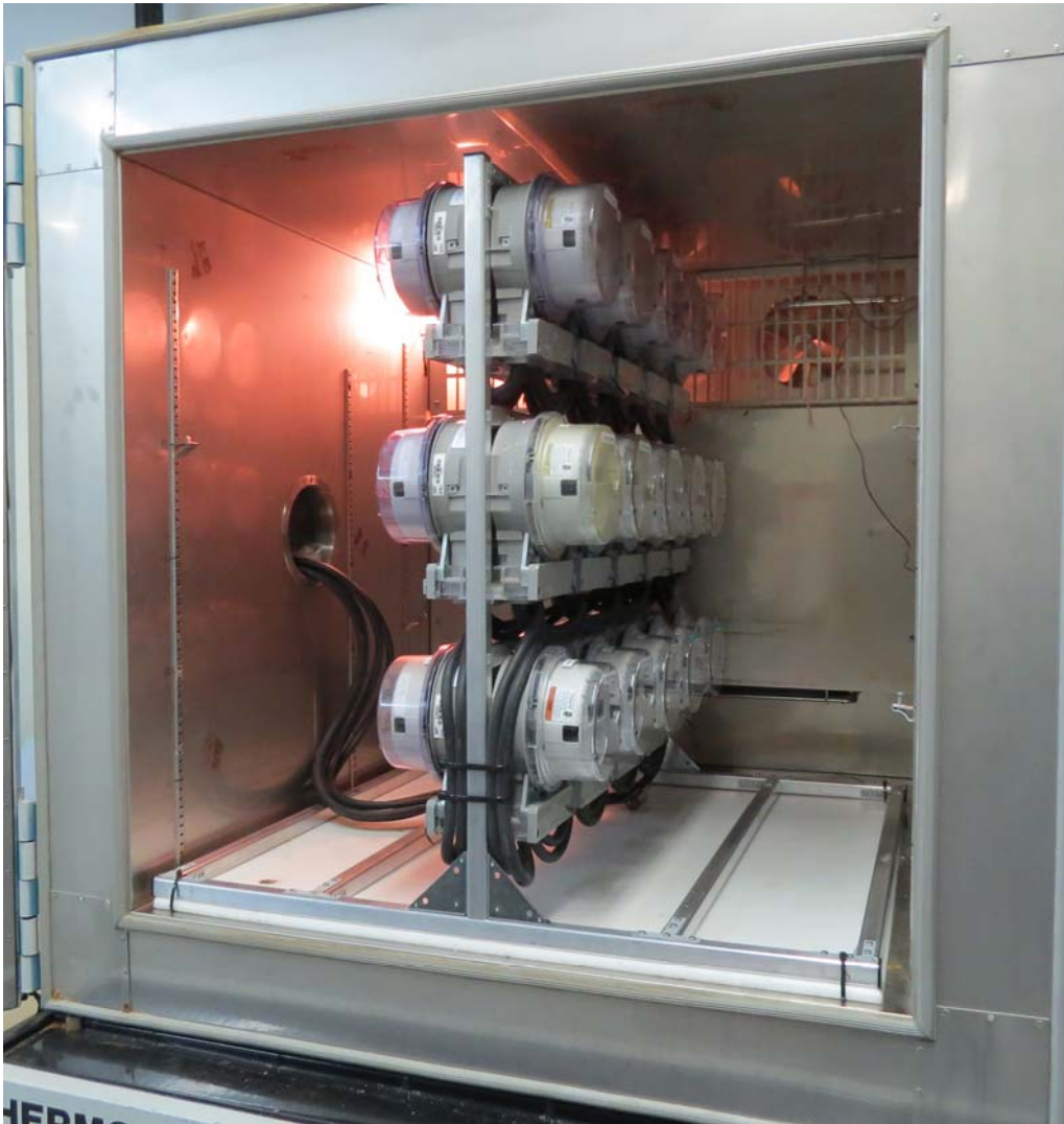
Figure 36. Meter testbed in environmental chamber for damp heat testing
