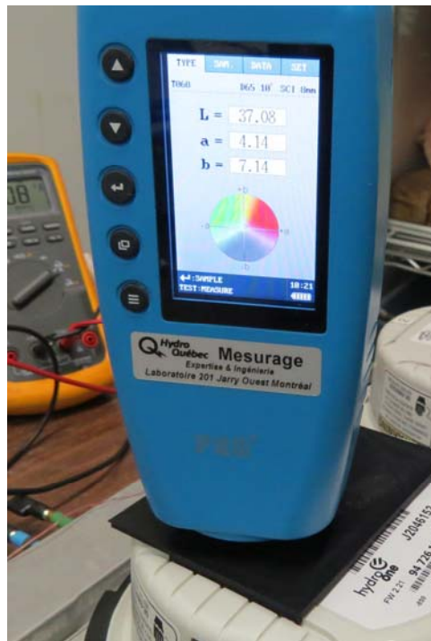
Figure 16. LCD colour measurement setup with template
