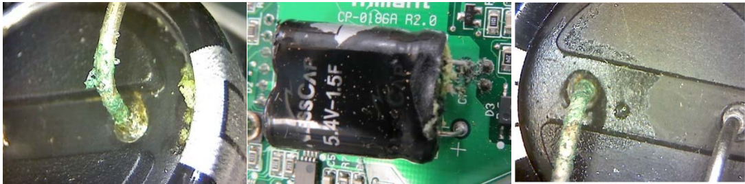
Figure 76: Capacitor Electrolyte Leakage
