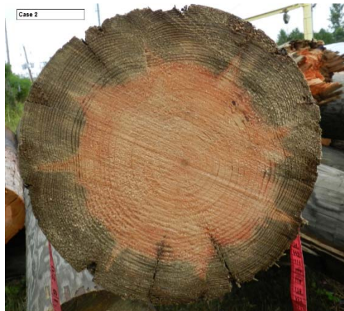
12 Figure 27: Treated Wood Pole Cross Section
