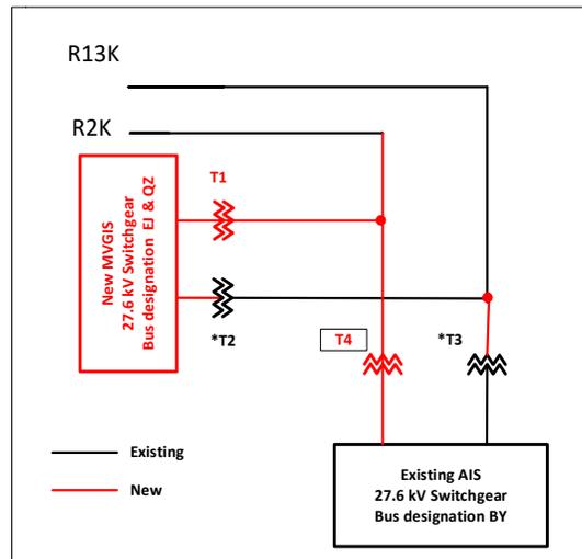
Figure 2- Horner TS: Proposed Facilities
