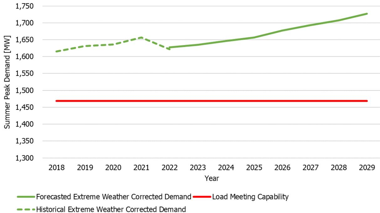
American Electric Reliability Corporation (NERC) TPL-001-5 planning standards. Based on this limiting contingency, the 2021 Addendum Study identified the load meeting capability (“LMC”) of the system supplying the Richview South area to be approximately 1,470 MW.
