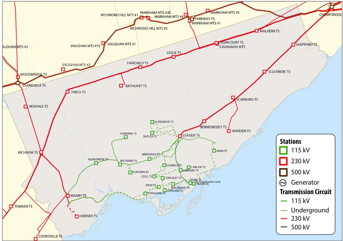
Figure 4-2: The Toronto Region Electrical System (Single-Line Diagram)
