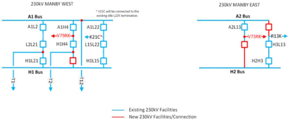
**Figure 3:Proposed Phase 2 Transmission Circuits Between Manby TS and Richview TS**
