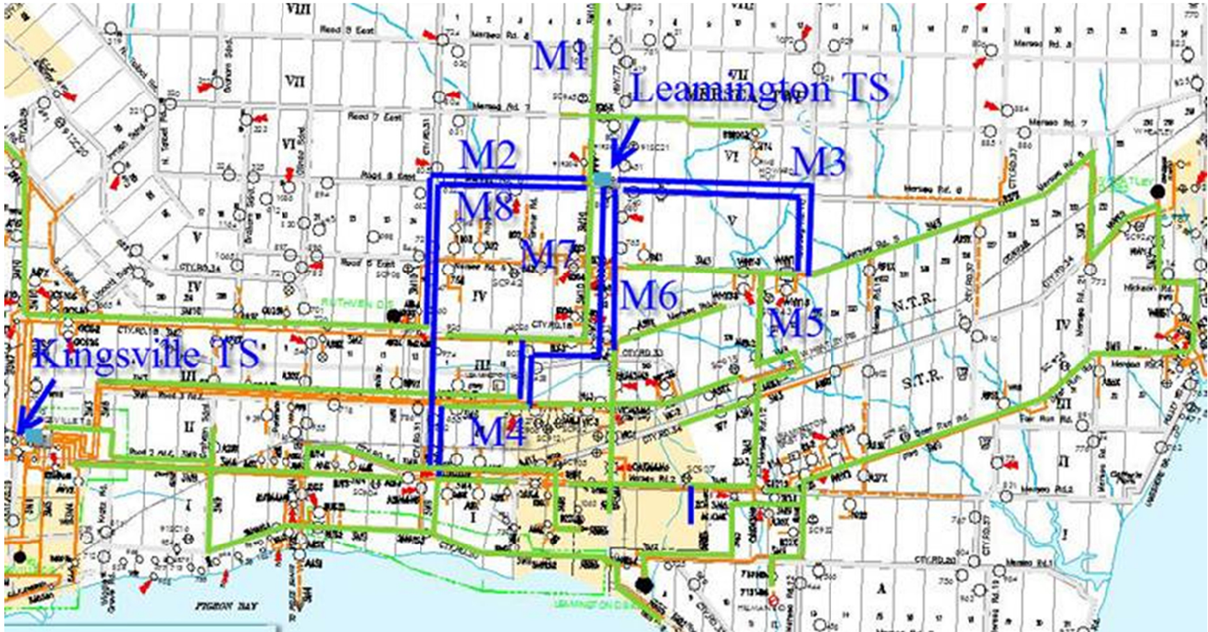
Figure 7-2 Preliminary Distribution Feeder Plans for SECTR Project
