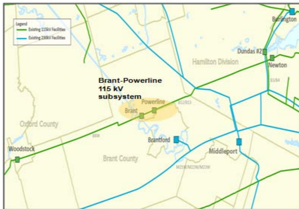
Figure 2-1: Brant Area Electricity System
