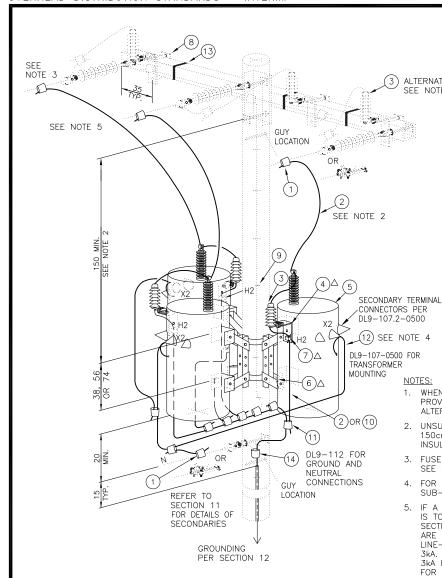
WHEN TRANSFORMER DOES NOT HAVE PROVISION FOR ARRESTER MOUNTING, USE ALTERNATE LOCATION.
