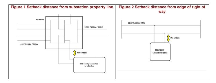
These setback distances achieve multiple purposes: allow safe operation of the grid, allow for maintaining, connecting, and expanding the transmission system or transformer station as needed, and reduce the potential for the BESS facility to
