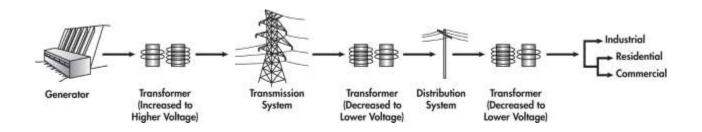
Transmission and distribution networks are sometimes referred to as the "electricity grid" or simply "the grid". For simplicity, the diagram above does not show customers directly connected to the transmission system or distributed generation sources or other distributors that may be connected to the distribution system.
