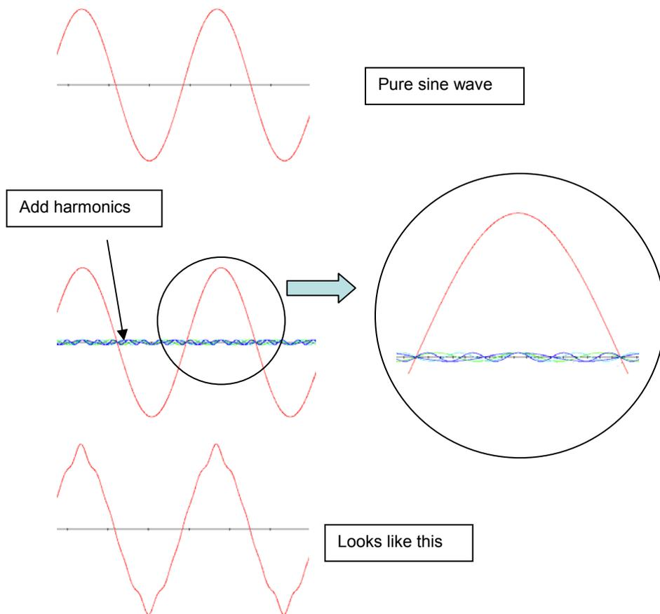
Harmonics can be measured through the use of power quality instruments. Excessive harmonics can impact the operation and performance of AC powered equipment.
