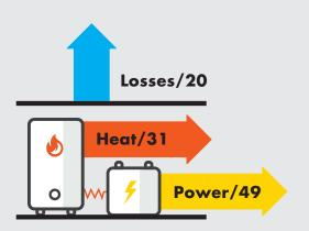
\*CHP is 80% efficient, which is about 47% more efficient than power and heat from separate sources.
