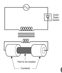
physically make contact with the product being heated. See diagram above. For food products, the sauce or gravy is the component that conducts the electric current, and the process is sometimes called "ohmic heating." The resistance (R) of the product to the flow of current (I) passing through it generates the I<sup>2</sup>R heating power. Low frequency current (60 Hz) heats the part throughout.High frequency current (400 kHz) tends to heat only the surface of the part.
