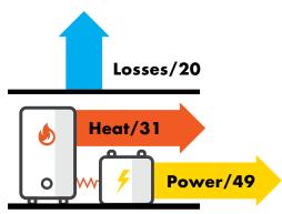
By transforming wasted heat into useful energy, a CHP system is up to 80% more efficient than traditional power generation.
