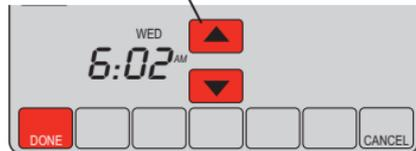
To set the current time display, press **CLOCK**, then press **▲** or **▼** to adjust the time. Press and hold **▲** or **▼** to advance the time more quickly.
