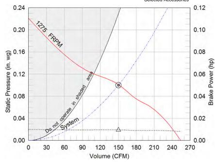
Operating Bhp point Operating point at Total SP Operating point at External SP Fan curve ---- System curve ----- Brake horsepower curve
