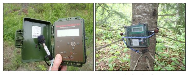
Figure 3. Wildlife Acoustic Song Meter SM4Bat ultrasonic recorder (left) and (right) deployed at the Wawa TS in May-June 2019.
