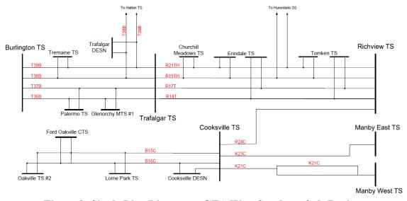
Figure 2: Single Line Diagram – GTA West Southern Sub-Region
