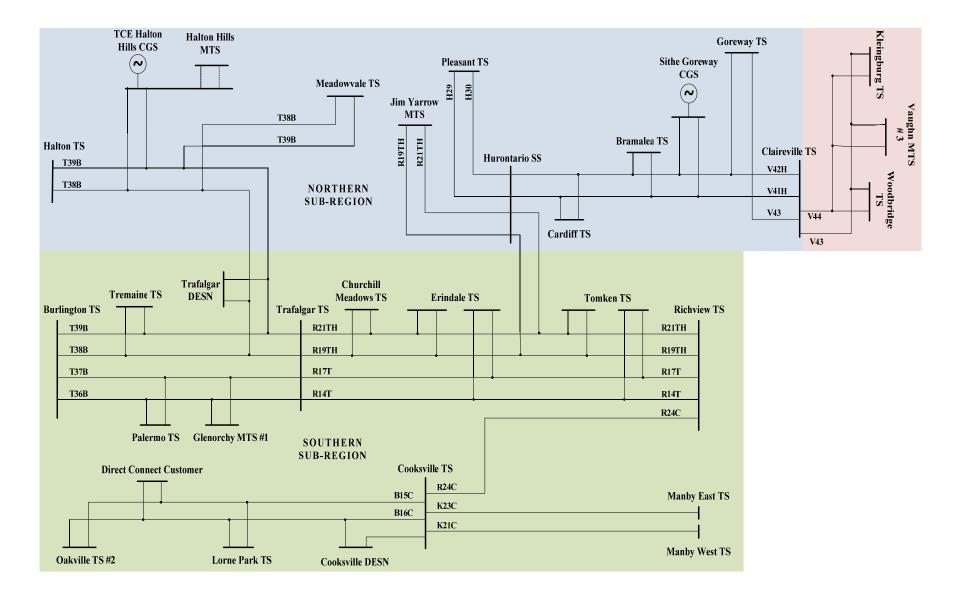
Figure 2: GTA WEST Region (Single Line Diagram)
