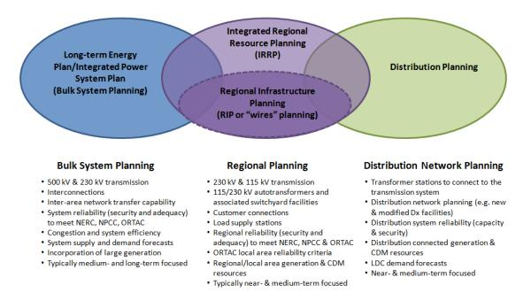
Planning at the bulk system level typically considers the 230 kV and 500 kV network. Bulk system planning considers the major transmission facilities and assesses the resources needed to adequately supply the province. Bulk system planning is carried out by the IESO in accordance with government policy. Distribution planning, which is carried out by local distribution companies, looks at specific investments on the low voltage, distribution system.
