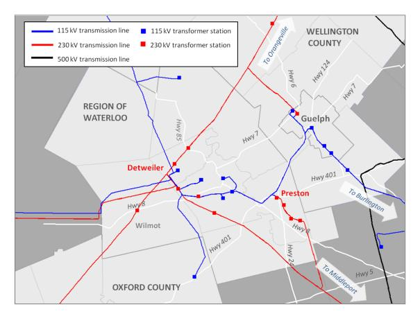
Along these local 230 kV and 115 kV networks, there are three transmission-connected customers and 25 step-down transformers that enable electricity to be delivered from the high-voltage transmission system (115 kV or 230 kV) to the low-voltage distribution systems that serve the communities.
