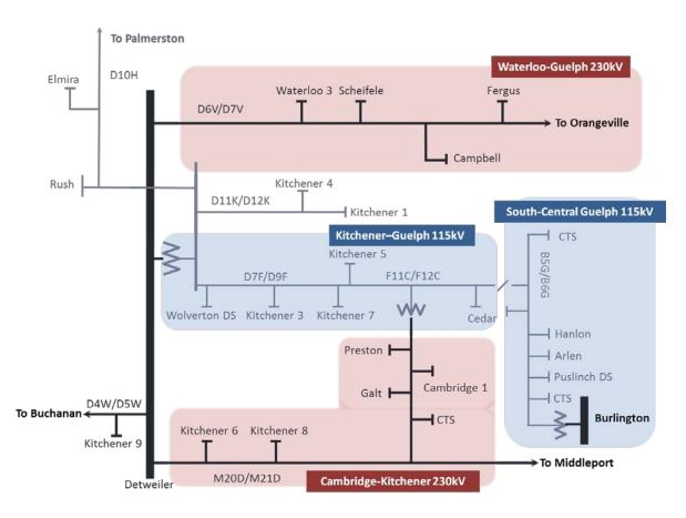
Today, the 115 kV sub-systems supplying the KWCG Region are at or approaching maximum capacity, and the 230 kV sub-systems have limited ability to restore electricity supply to customers in the event of a major transmission outage. Table 6-1 provides a summary of the near- and medium-term needs in the KWCG Region.
