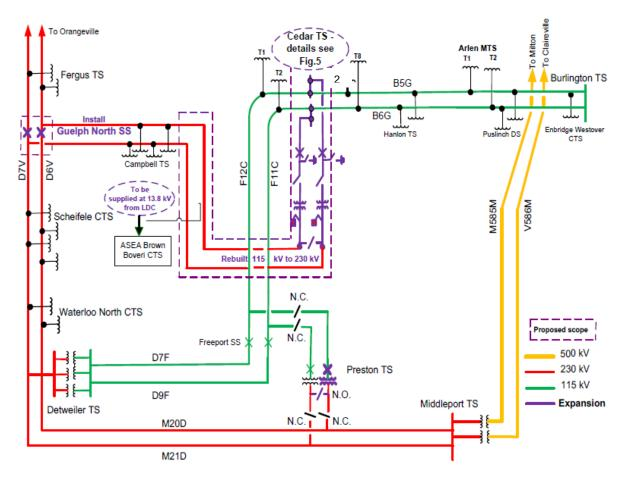
**Figure 1 :** Install two 230/115 kV autotransformers at Cedar TS, 2 in-line breakers at Guelph North Junction and 2 in-line breakers at Cedar TS
