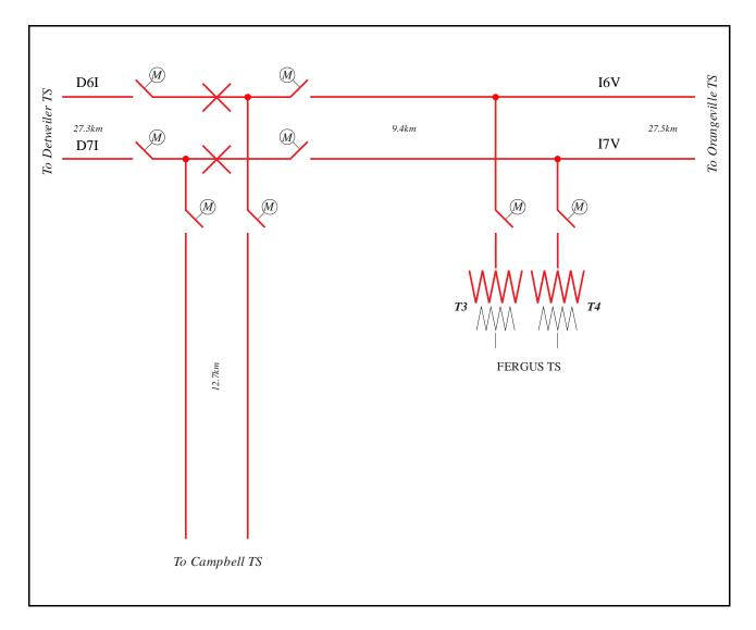
Figure 3: Hydro One Proposed Inverhaugh SS Station Configuration
