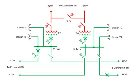
Figure 2 – Configuration of 2 in-line breakers (staggered) at Cedar TS Two 230 kV breakers at Guelph North Junction
