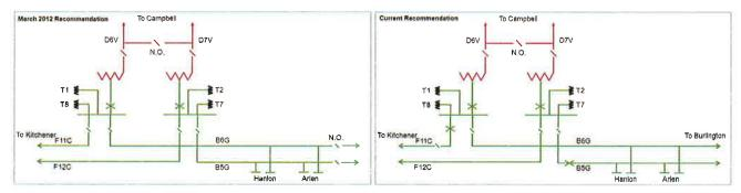
Figure 1. Cedar TS Switching Arrangement: Recommended Scope March 2012 and Current Recommendation
