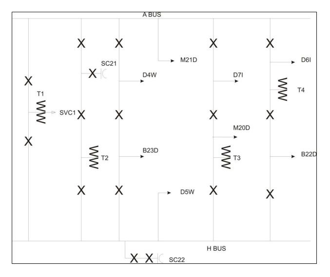
Figure 5: Detweiler 230 kV Station Configuration
