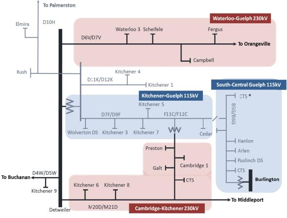
Figure 3-2 KWCG Single Line Diagram
