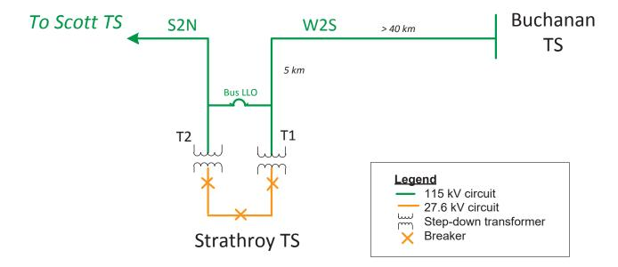
Figure 2 – Simplified schematic of Strathroy TS
