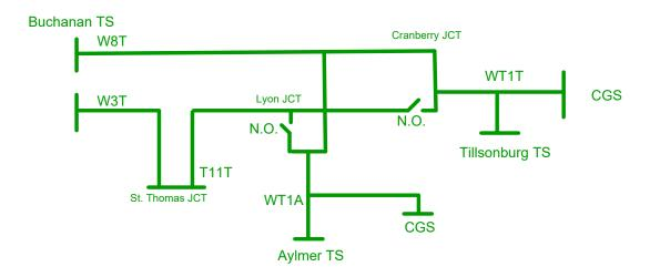
Figure 7-1 Existing Single Line Diagram of Aylmer-Tillsonburg Sub-Region
