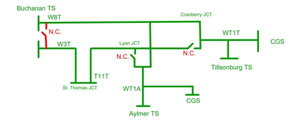
Figure 7-2 Single Line Diagram of Aylmer-Tillsonburg Sub-Region after Reconfiguration
