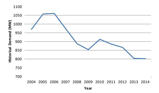
Peak demand in the Kingsville-Leamington area has experienced fluctuations comparable to the Region since 2004, which is shown in Figure 5-2 below. In addition to the trends described above, this figure shows the impact of approximately 16 MW of effective capacity of DG connected at Kingsville TS by 2015, none of which was connected in 2004.
