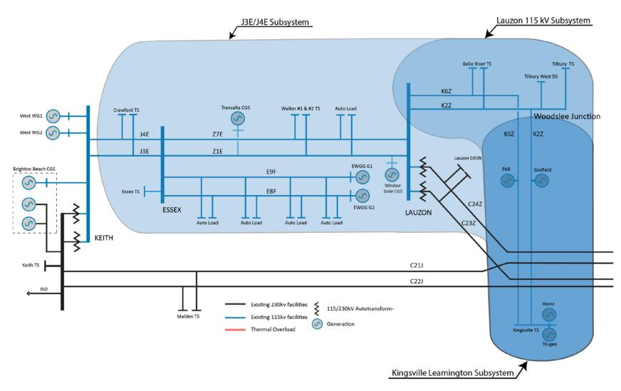
Figure 2. Windsor-Essex Region Subsystems/Single Line Diagram
