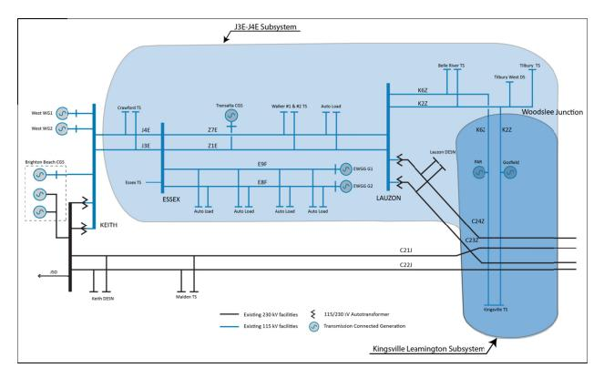
Figure 3-2 Windsor-Essex Area Subsystems/Single Line Diagram
