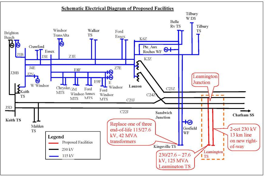
Figure 7-1 Schematic Electrical Diagram of the Proposed Facilities
