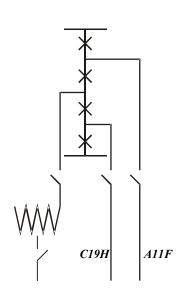
Typical Physical Arrangement for a Breaker-and-a-Third Layouts
