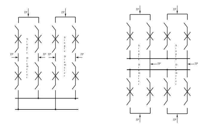
TP = Termination Point for a transmission element such as a circuit, transformer, etc.
