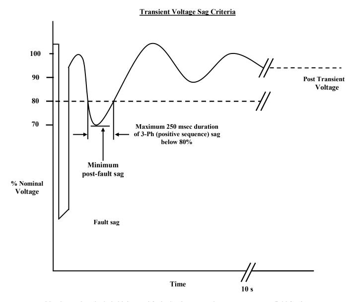
Mitigation options include high-speed fault clearing, *special protection systems*, field forcing, transmission reinforcements and transmission interface transfer limits.
