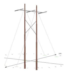
Figure 2: Two-Pole Dead End Structure.
