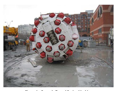
Figure 4 – Example Tunnel Boring Machine
