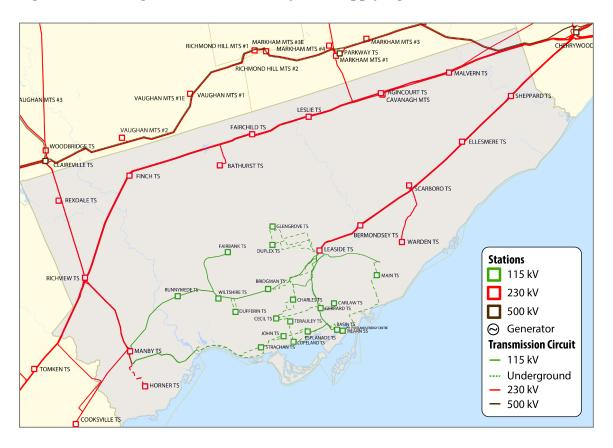
Figure 4-1: The Regional Transmission System Supplying Toronto
