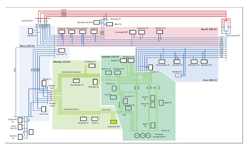
Figure 3-1: Single Line Diagram of Toronto Region's Transmission Network
