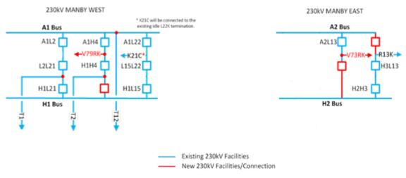
Figure 3: Proposed Phase 2 Transmission Circuits Between Manby TS and Richview TS
