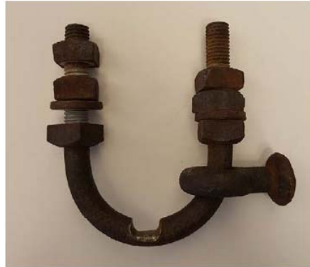
Figure 54 - A Worn U-bolt
