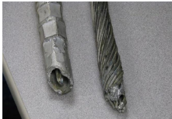
Figure 2 - Broken ACSR Conductor
