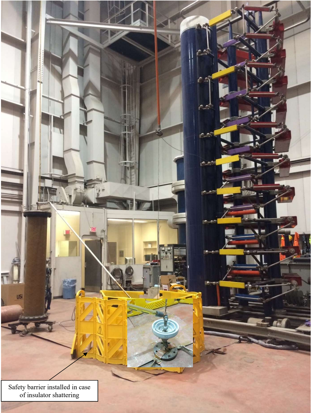
Figure B-9 Step front test setup
