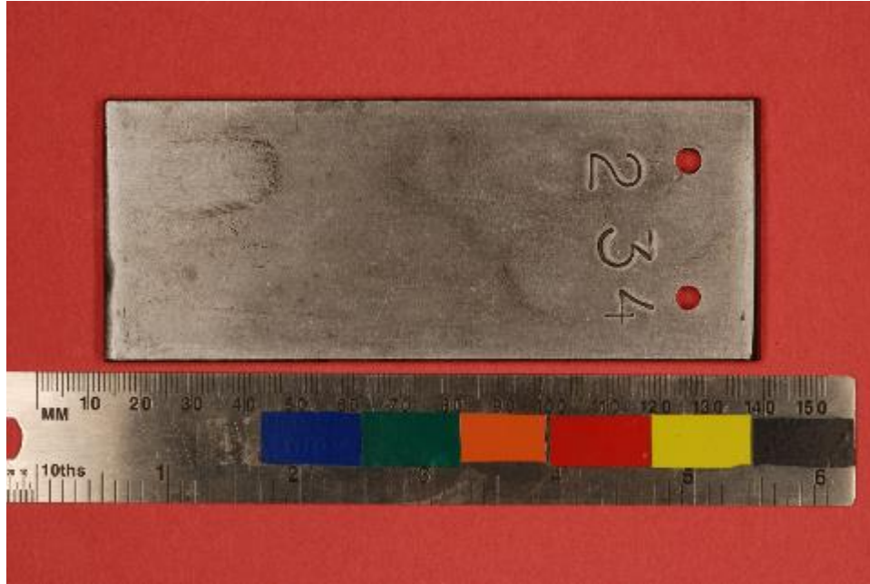
Figure 2-2: Bare Carbon Steel Coupon That Has Been Serialized, Weighed, Measured and Characterized by Color
