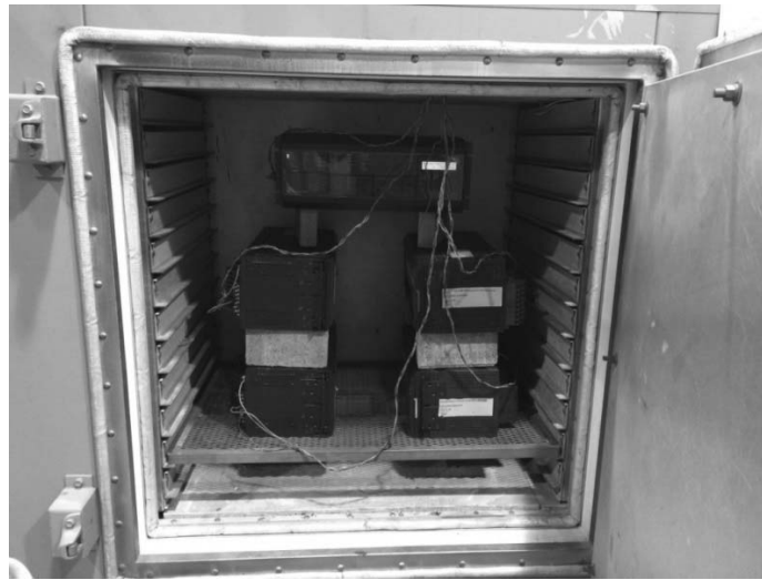
Figure 4-2: D60 Relays in Oven
