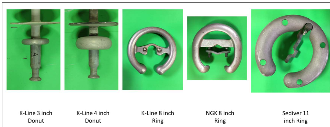
Figure 2-6 Various corona rings present on sample insulators
