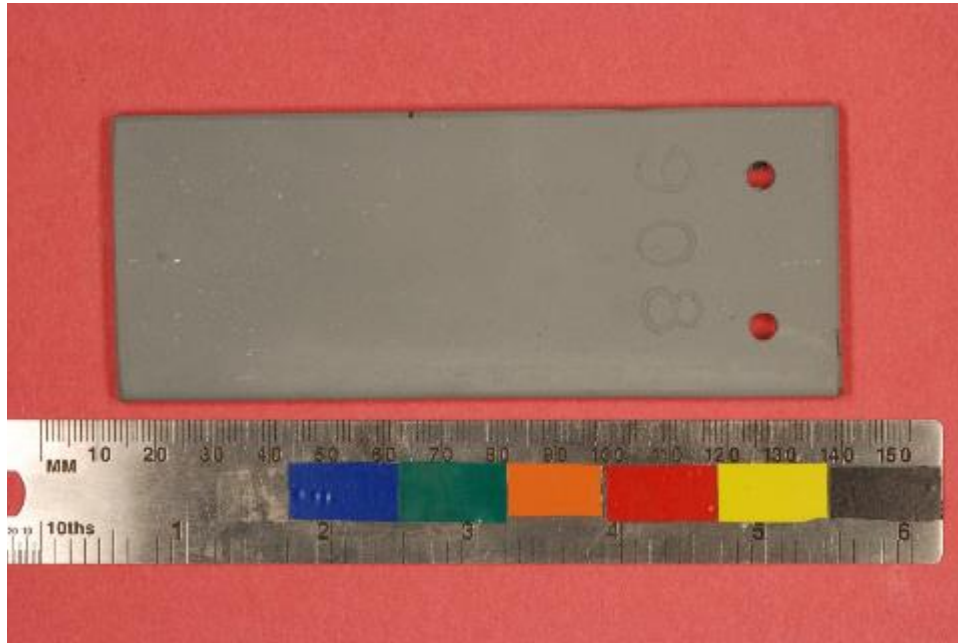
Figure 2-4: Coated Steel Coupon That Has Been Serialized, Weighed, Measured and Characterized by Color
