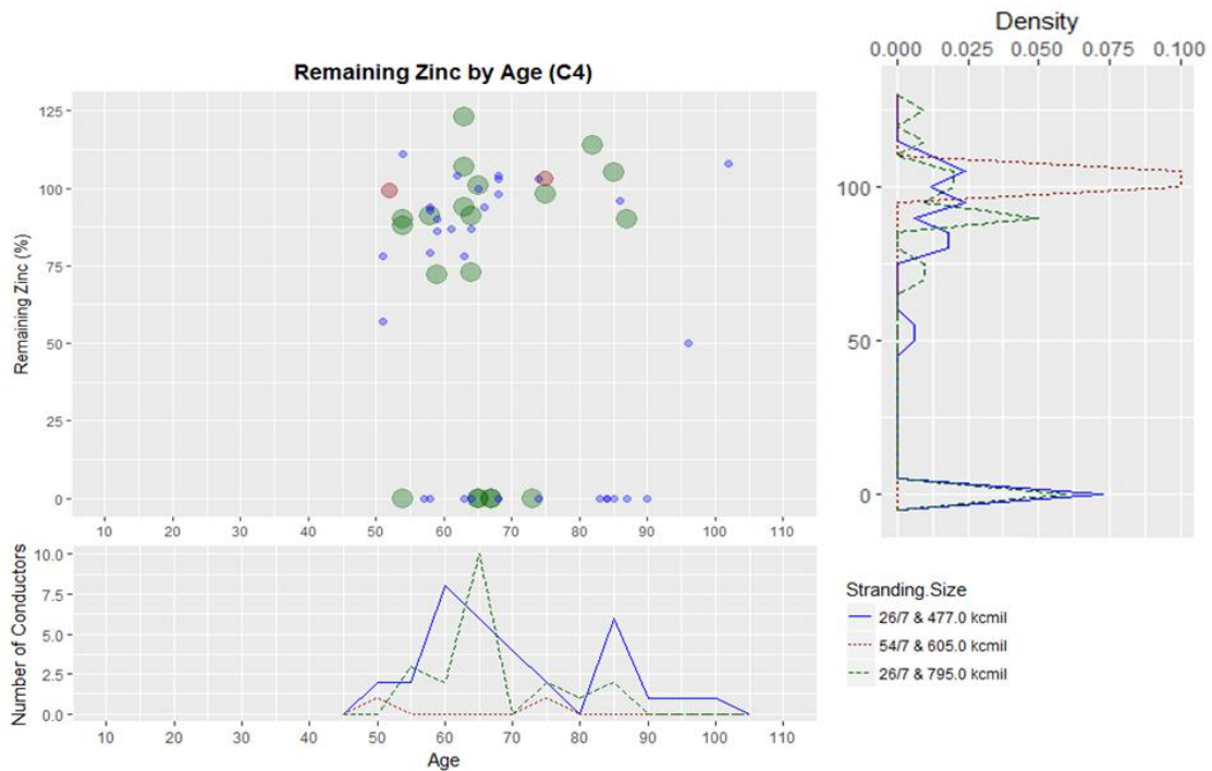
Figure 3-50 Remaining Zinc by Age: Corrosion Zone C4
