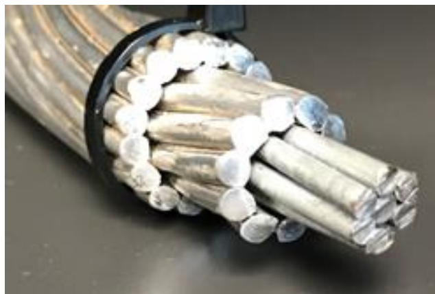
Figure 1-2 Aluminum Conductor Steel Reinforced (ACSR 26/7 Drake)
