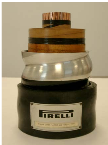
Figure 2.4 Cross-section of LPLF cable
