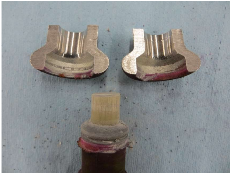
Figure 4-13 Dye entering the end fitting through a compromised secondary seal but not reaching the fiberglass rod
