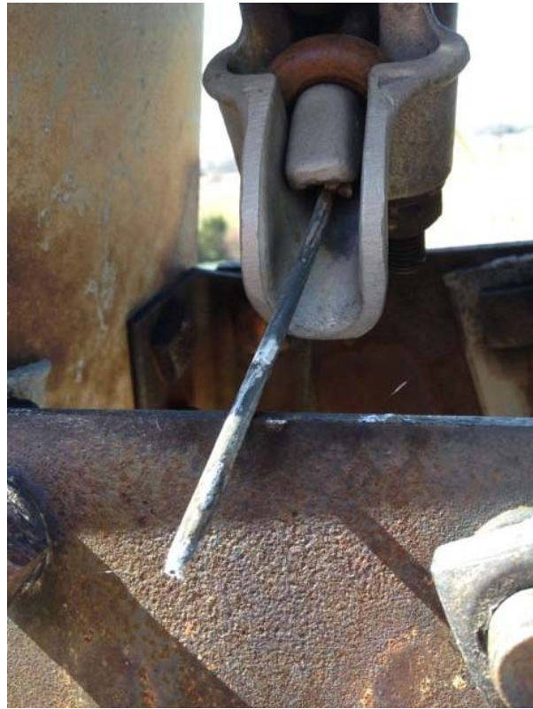
Figure 3: 2016 Shieldwire Failure on K2Z
