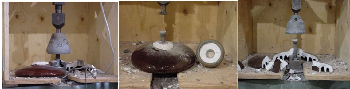
Figure B-5 Typical modes of failure observed with the aged population of insulators being investigated
