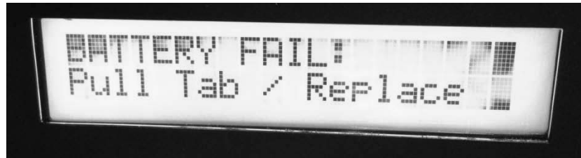
Figure 6-1: Example of Darkening of D60 LCD
