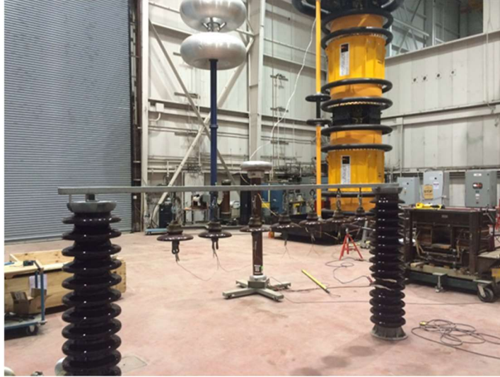
Figure B-3 Insulators undergoing ac withstand test
