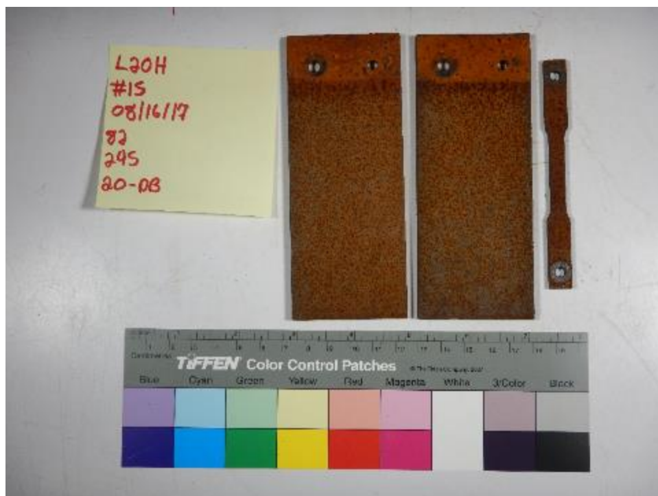
Figure 2-8 Image record for each coupon with color correction
