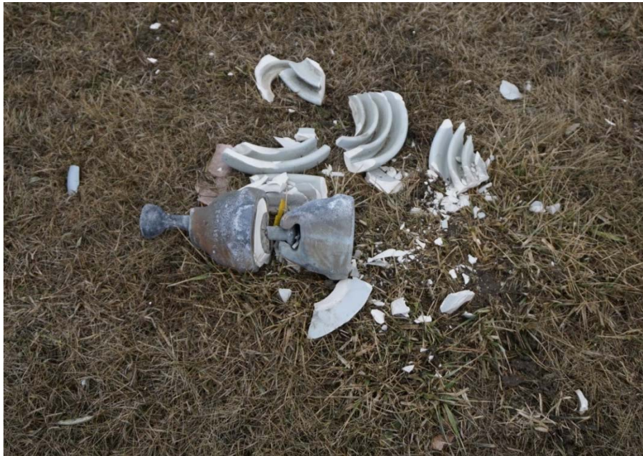
Figure 37 - V76R Insulator Failure
