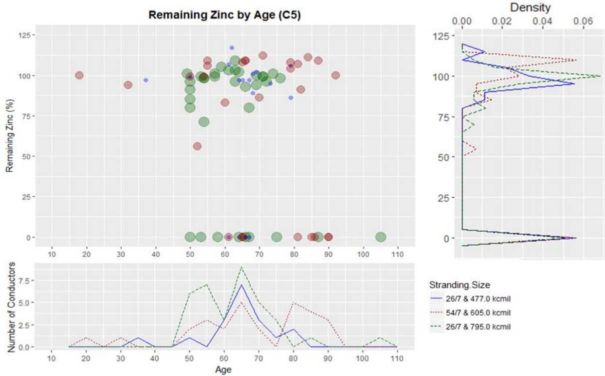
Figure 3-51 Remaining Zinc by Age: Corrosion Zone C5
