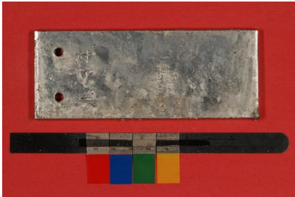
Figure 2-3: Galvanized Test Coupon That Has Been Serialized, Weighed, Measured and Characterized by Color
