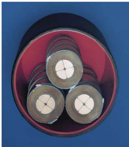
Figure 2.1 Cross-section of HPLF cable
