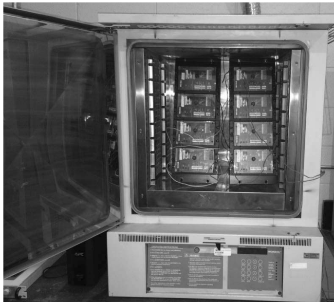
Figure 4-1: MCGG 22 Relays in Oven
