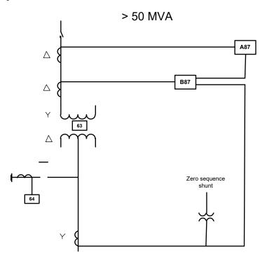
Figure 4 - 64 Ground Connected Overcurrent
