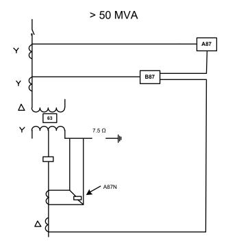
Figure 5 - A87N Transformer Protection
