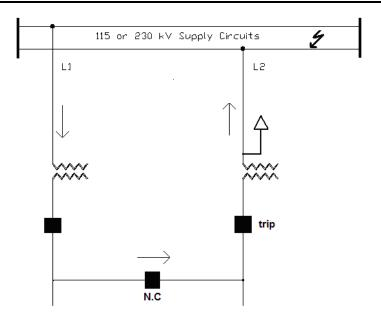
Figure 2 - Line Backup Protection Required – Transformers in Parallel
