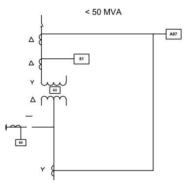
Figure 6 - Transformer 51 Protection
