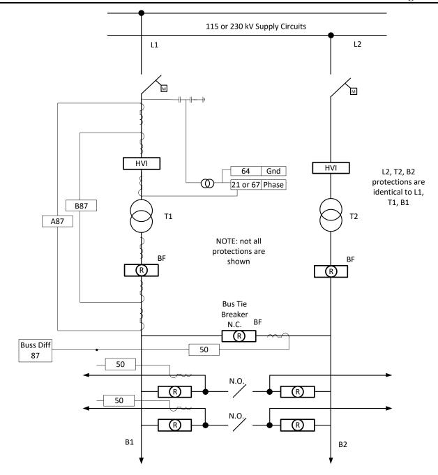
Figure 8 - DESN Load Connection Facility with HVI
