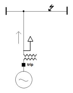
Figure 3 - Line Backup Protection Required - Large MMF exists on Low Voltage Bus
