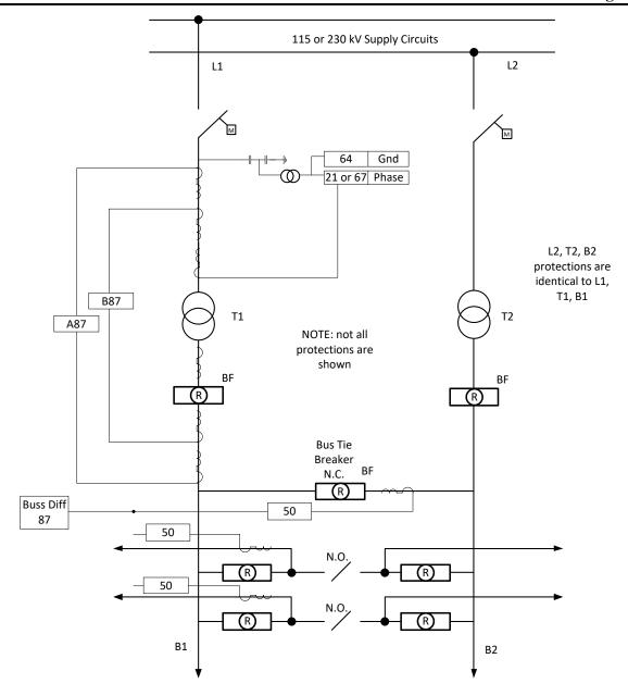
Figure 7 - DESN Load Connection Facility with no HVI
